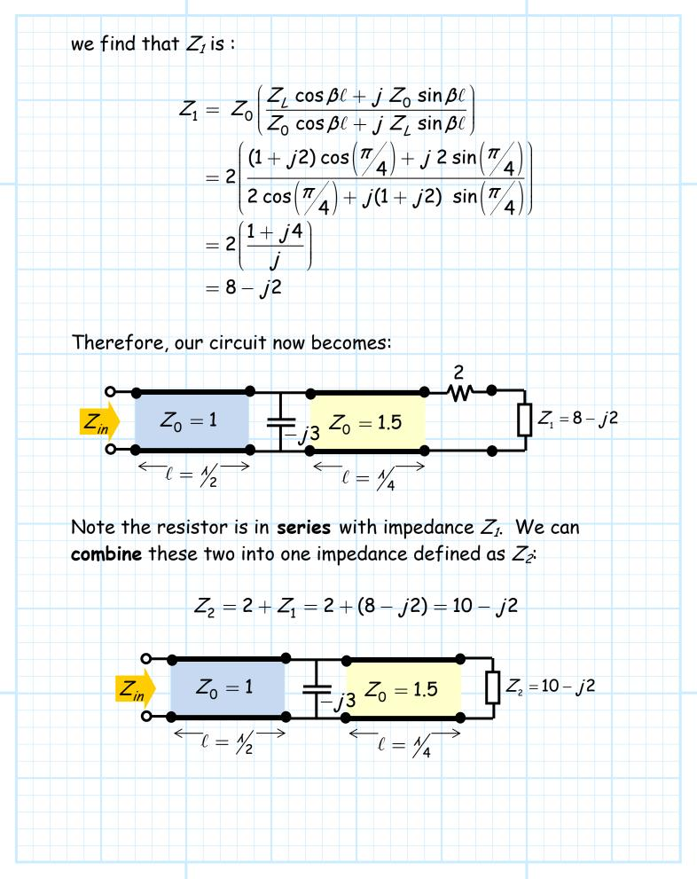
Now let's define the input impedance of the **middle** transmission line section as  $Z_3$ :
